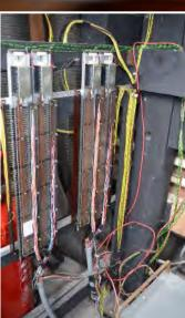
The switches for the pedal stops are corroded and the wiring in a poor state.
